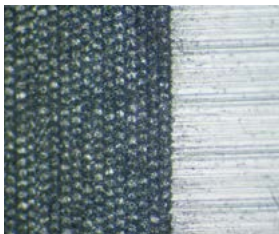
Pre-welding surface processing
