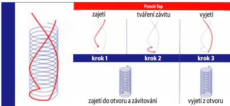
Obr. 4: Kinematika technologie Punch Tap
